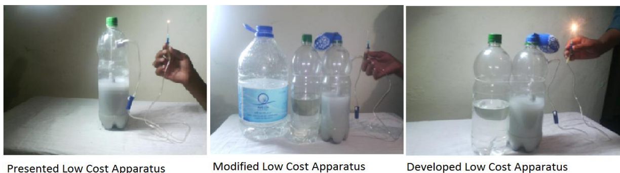
Figure 3.1. Low Cost Apparatus for the Preparation of Acetylene Gas
