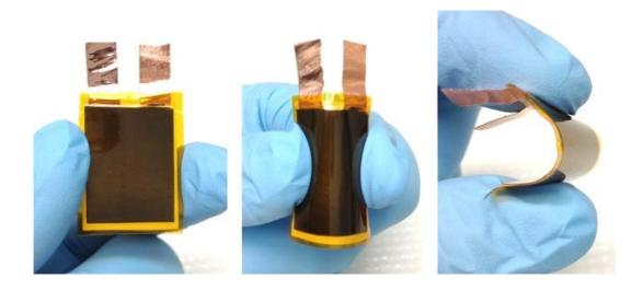
• Novel thienothiophene polymer and its synthesis method for electrochromic and flexible supercapacitor applications
